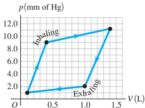
Figure 1: pV-diagram.
