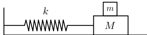
Figure 2: If the amplitude is large enough the block on top will slide.
