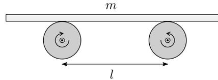
Figure 5: A rod oscillating between the wheels.
