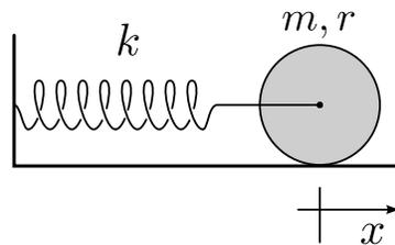
Figure 1: The oscillation with rolling.
