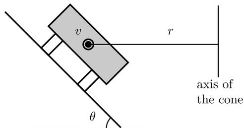
Figure 2: A car turning on a curved surface of a cone.
